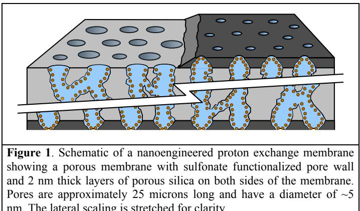
**Figure 1.** Schematic of a nanoengineered proton exchange membrane showing a porous membrane with sulfonate functionalized pore wall and 2 nm thick layers of porous silica on both sides of the membrane. Pores are approximately 25 microns long and have a diameter of ~5 nm. The lateral scaling is stretched for clarity.
