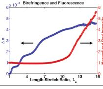
Representative birefringence ( $\Delta n$ ) and fluorescence (red intensity normalized by first image red intensity) averaged over the gauge section of a PMA-SP-PMA tensile specimen vs. the length stretch ratio ( $\lambda_s = L_{current}/L_o$ ), indicating a need for moderate polymer chain alignment (significant birefringence) before activation of the SP (increase in fluorescence).
