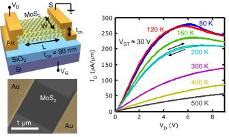
drift velocity shows usual saturation behavior (vsat  $\approx 2 \times 106$  cm/s at 300 K). Comparisons with electro-thermal and Boltzmann transport simulations reveal this behavior is caused by a combination of self-heating and transport through multiple conduction bands. Such results have not been previously observed in twodimensional semiconductors and provide key insights into the effect of their complex band structure on practical device operation.
